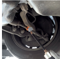
Releases steering linkage
