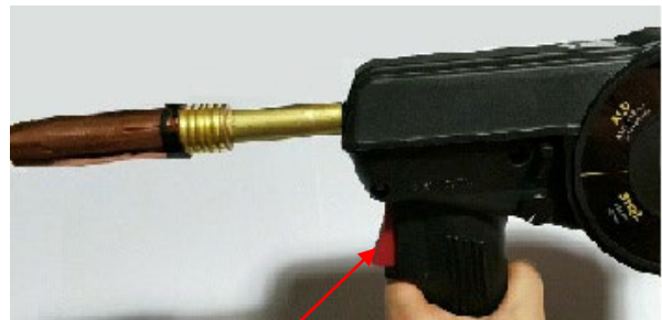
(11) Pull the trigger to drive the wire down the neck until it exits the contact tip.
