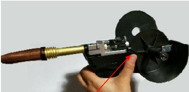
(8) Remove the spool cover by pressing button and lifting off the cover.
