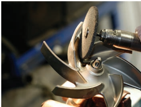
Finishing, maintaining and repairing turbine and propeller blades, without affecting their geometry.
