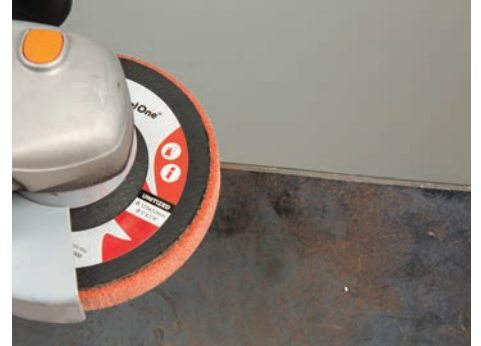
Breaking angles, deburring and rounding.
