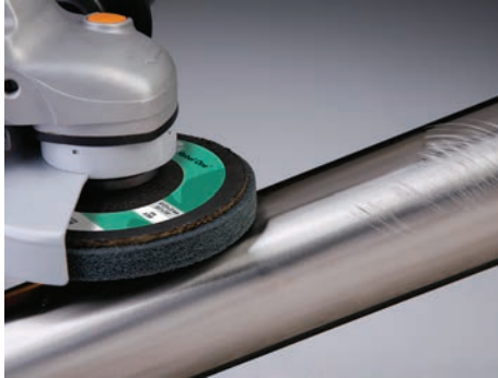
Correcting sanding errors, removing scratches.
