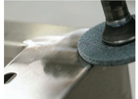
Improving surface roughness. Controlling the Ra value.
