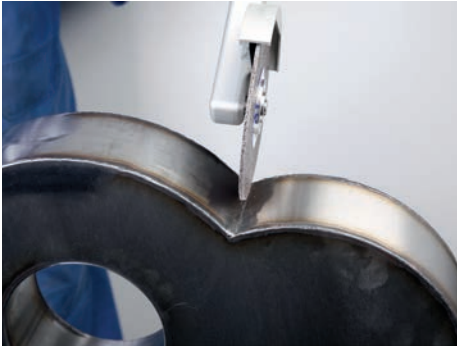
Removing TIG welds.
